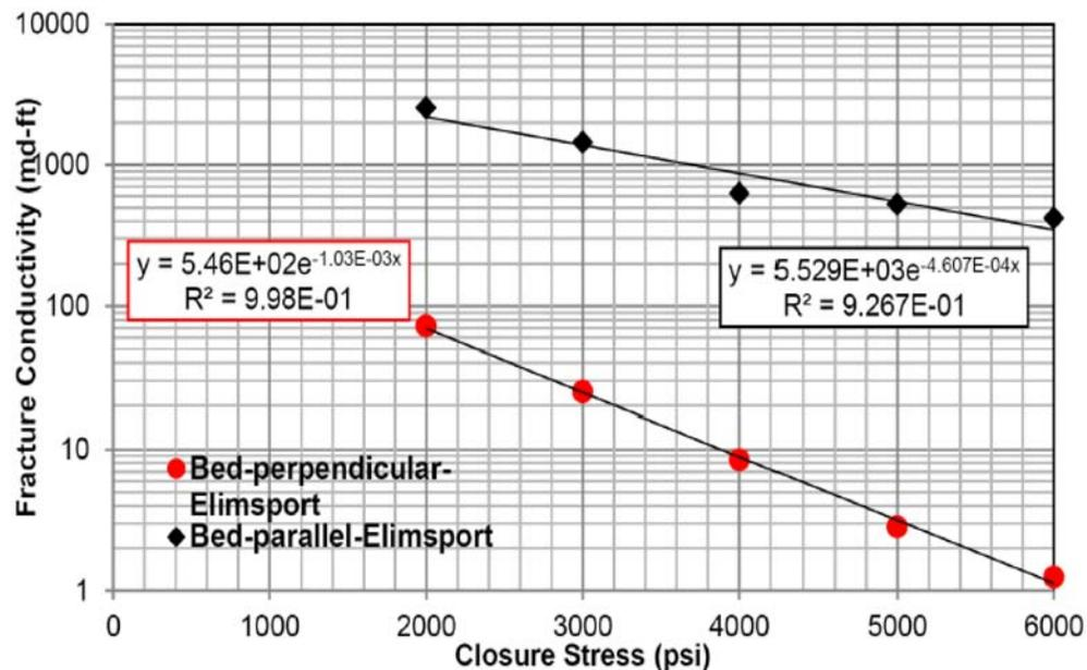
Figure 2—Measured Propped Fracture Conductivity versus Closure Stress for Elmsport Samples (McGinley et al., 2015)
