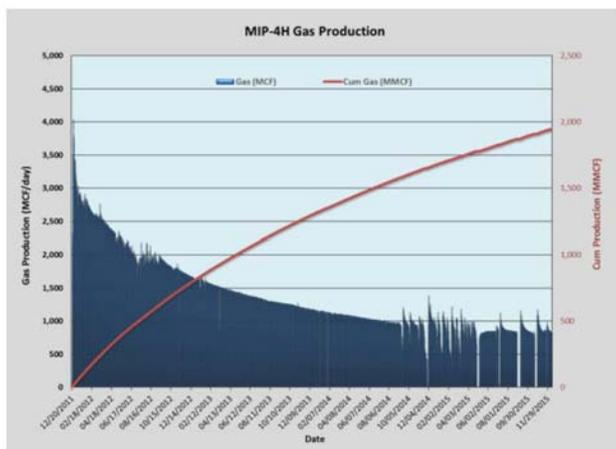
Figure 9—The production and cumulative production for MIP-4H
