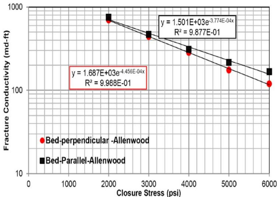
Figure 3—Measured Propped Fracture Conductivity versus Closure Stress for Allenwood Samples (McGinley et al., 2015)
