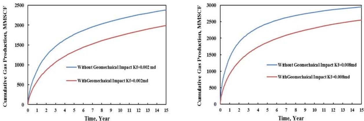
Figure 16—Impact fissure permeability on stress-dependent propped hydraulic fracture conductivity for cumulative gas production
