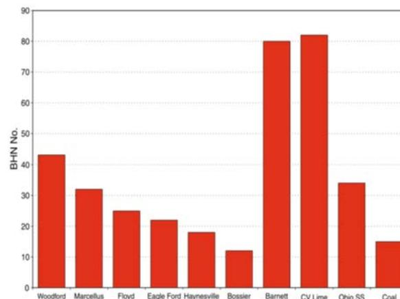
Figure 1—Brunell Hardness Numbers for various shale reservoirs in North America ([Stegent et al., 2010](#)).
