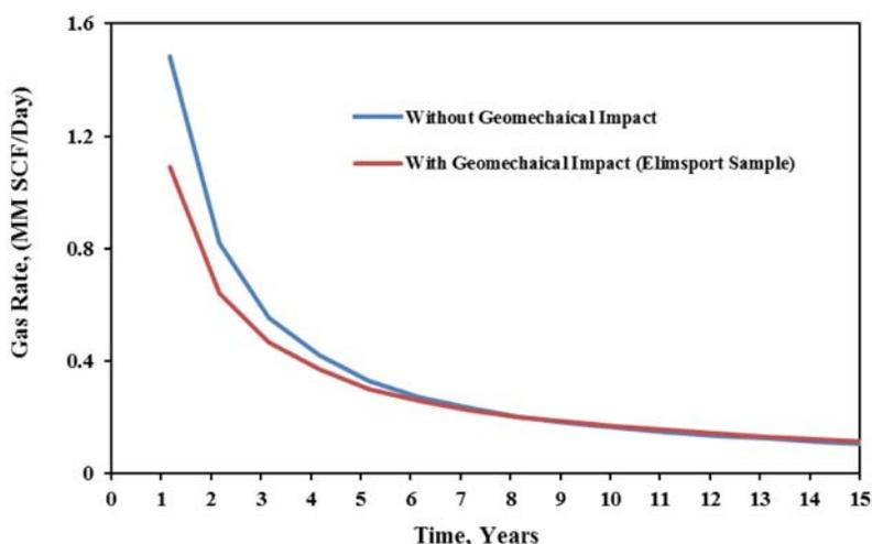
Figure 13—Gas flow rate for 15 years with and without considering geomechanical effect for MIP-6H Well (Elimsport Sample)
