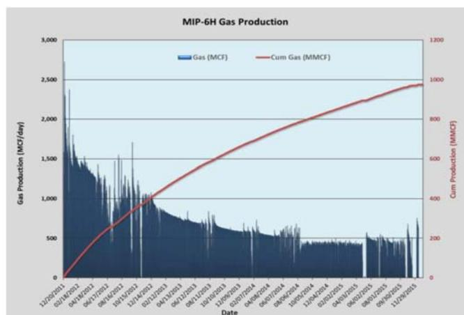
Figure 10—The production and cumulative production for MIP-6H
