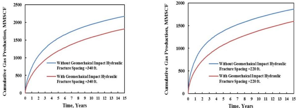
Figure 19—Impact hydraulic fracture spacing on stress-dependent propped hydraulic fracture conductivity for cumulative gas production
