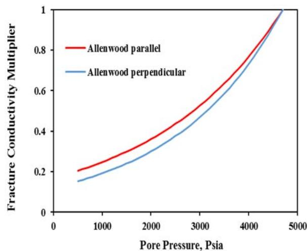
Figure 5—Fracture Conductivity Multiplier for Allenwood Sample
