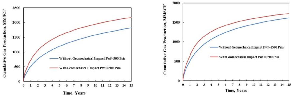
Figure 15—Impact Pwf on stress-dependent propped hydraulic fracture conductivity for cumulative gas production
