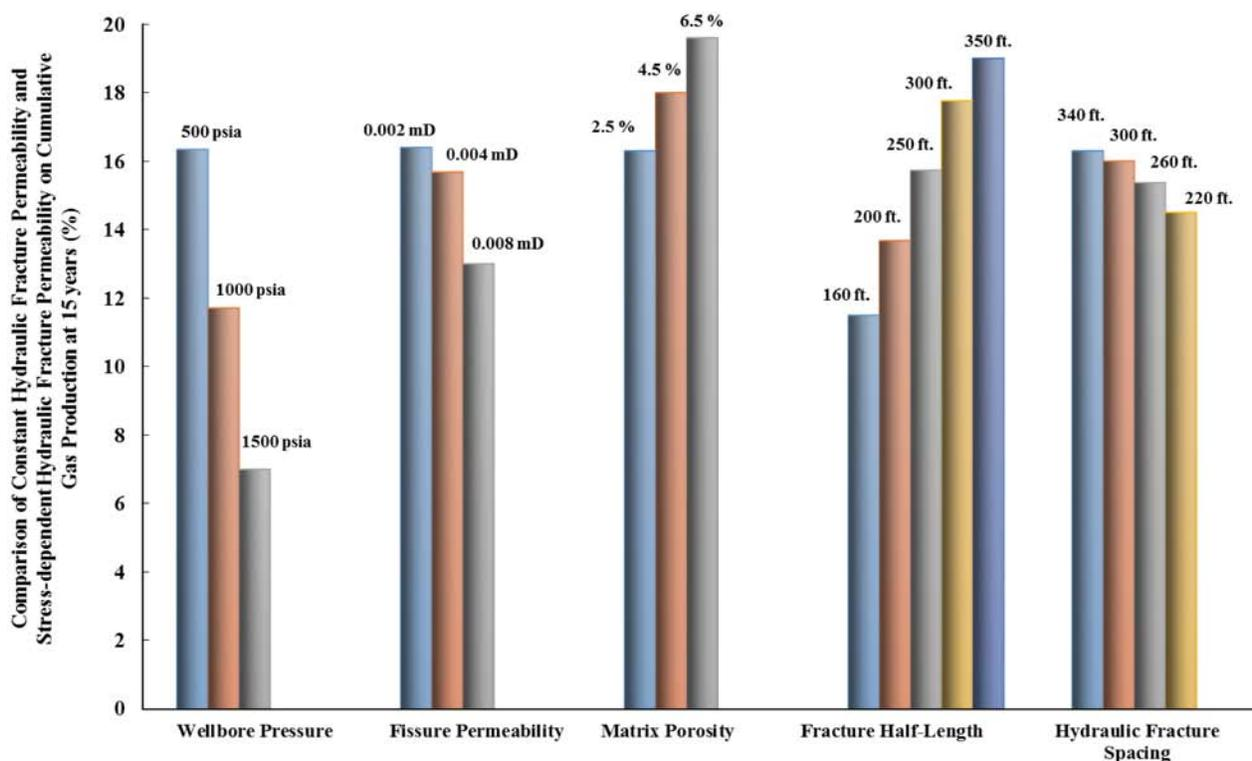
Figure 20—Illustrates critical parameters that influence the stress-dependent propped hydraulic fracture conductivity
