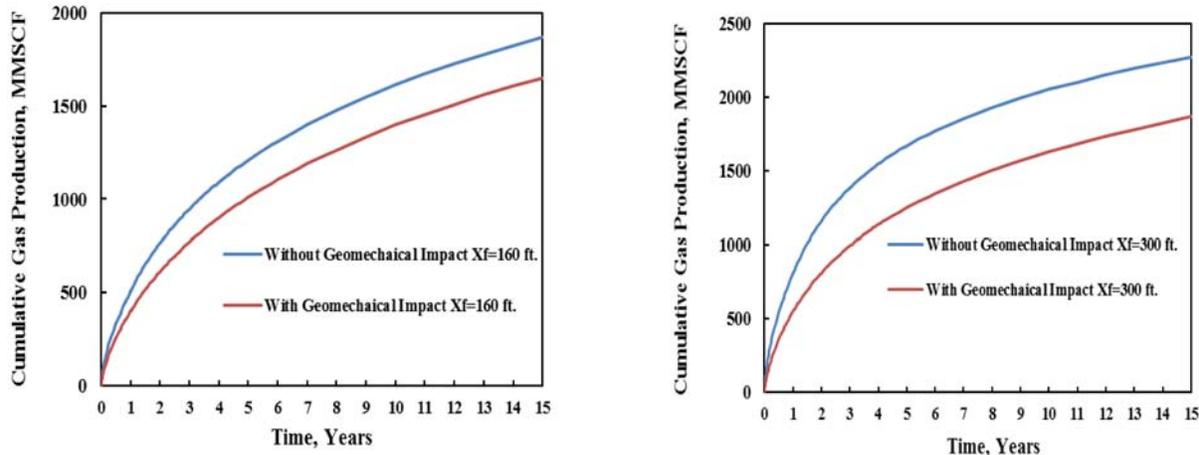
Figure 18—Impact fracture half-length on stress-dependent propped hydraulic fracture conductivity for cumulative gas production
