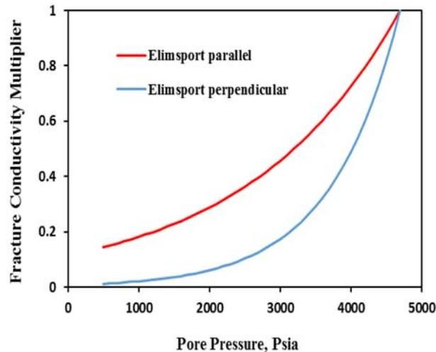
Figure 4—Fracture Conductivity Multiplier for Elimsport Sample
