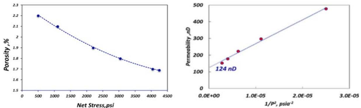
Figure 7—Porosity and Permeability from core plug (Elsaig et al., 2016)
