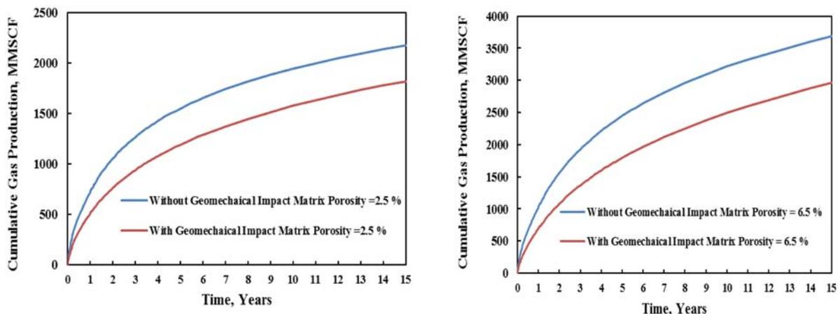
Figure 17—Impact matrix porosity on stress-dependent propped hydraulic fracture conductivity for cumulative gas production
