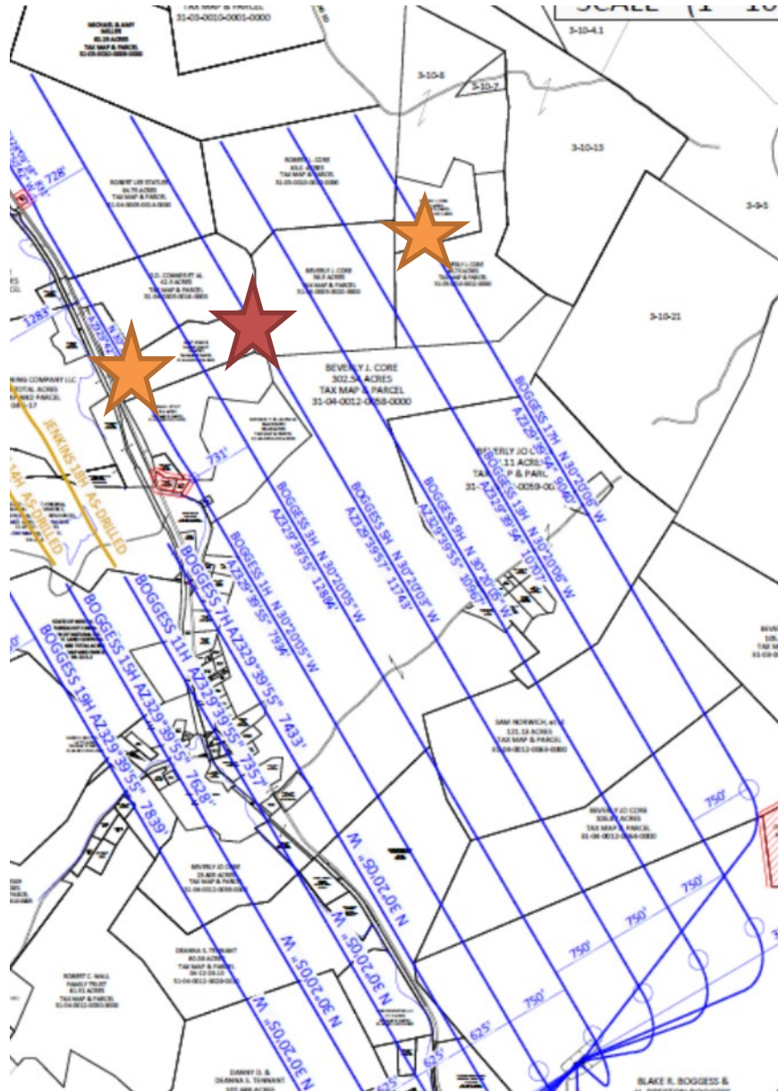
Figure 1.1: Boggess Pad with new generation permanent fiber in the central well (Boggess 5H, red star) and deployable fiber in adjoining wells skipping one (orange stars). We will be able to monitor in near-real time fracture stimulation in the central 3 wells (3H, 5H and 9H). A vertical pilot will be drilled, cored, and logged.
