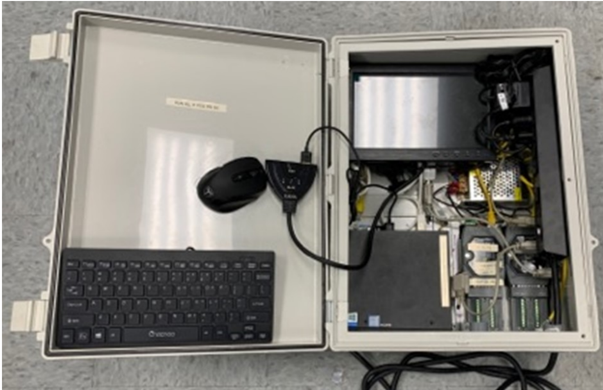
Figure 5.2: Final DAQ system for energy audits.
