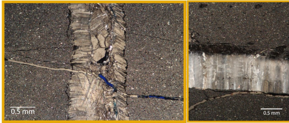
Figure 1.2: Examples of the numerous calcite and bitumen filled fractures observed in the core from the MIP 3H pilot well. These fractures appear to influence hydraulic fracture stimulation efficiency.
