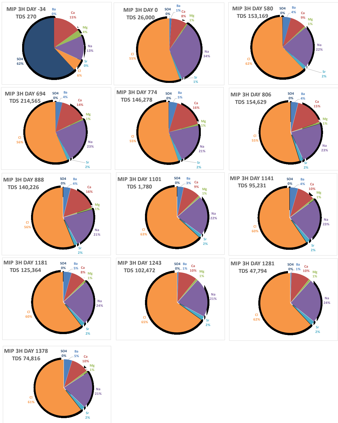
Figure 4.1. Changes in major ion concentrations in produced water from well MIP 3H. Top left Day -34 represents makeup water from the Monongahela River, top center is produced water on the first day (Day 0) and the remainder of pie charts show flowback and produced water on sampling dates through the 1378th day post completion.
