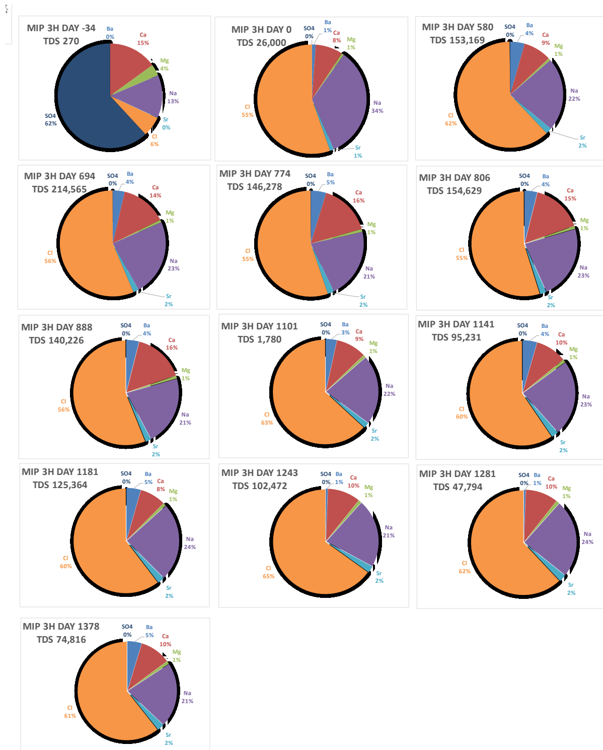
Figure 4.1). While produced water TDS (total dissolved solids) increased by an order of magnitude from initial flowback to the present, the ionic composition of produced water changed very little through 1281 days post completion. Produced water TDS was affected by shut-in/turn-in cycles at individual wells. For example, upon turn-in TDS was invariably very low but reached pre-shut-in concentrations within a month.
