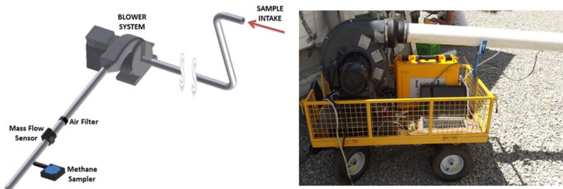
Figure 5.1. WVU's Full Flow Sampling System
