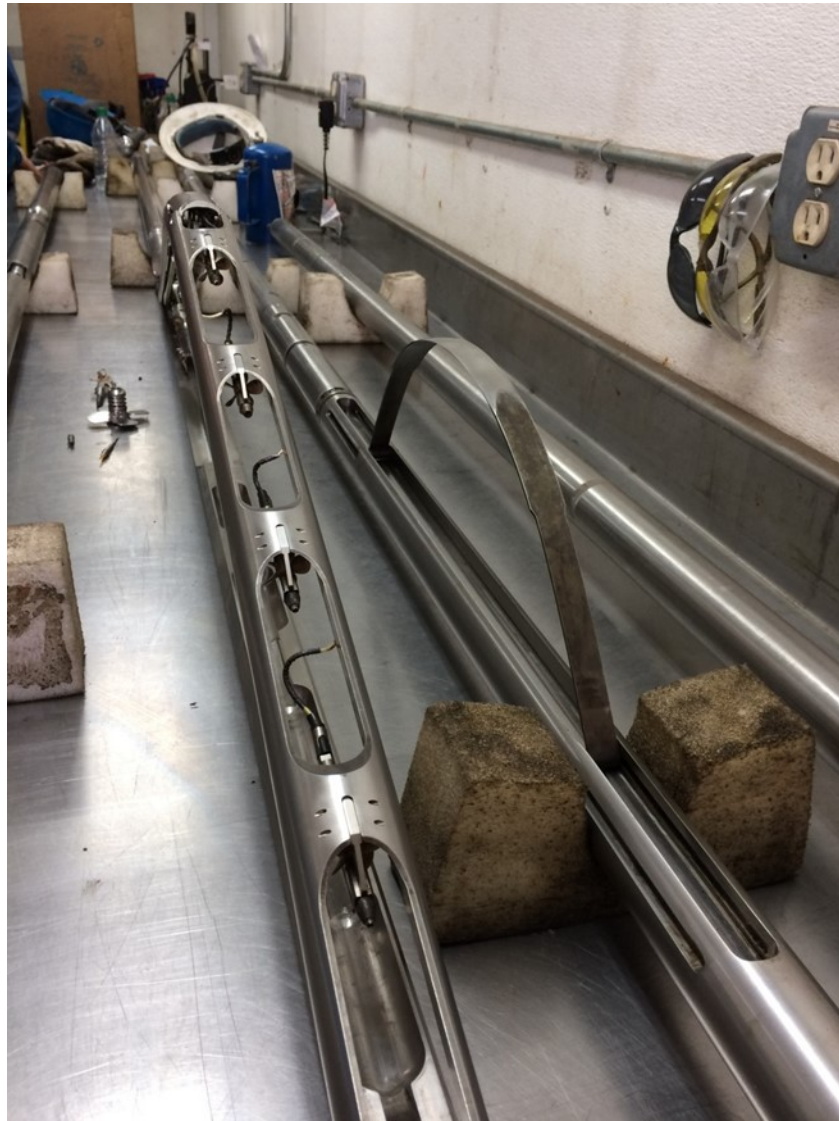
Figure 1.1, Schlumberger's Flow Scanner logging tool before deployment in the MIP 3H showing spinners and other tool components. Tool expands to measure flow at different level in the lateral.
