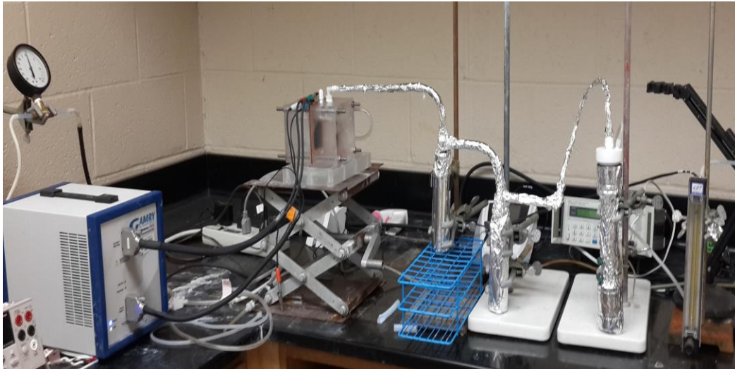
Figure 2.b.1. The two-chambered electrolysis system for generating high-pH catholyte.
