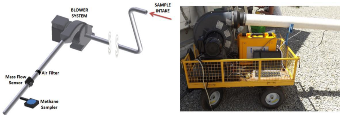
Figure 5.b.1: Left- schematic of FFS, Right- image of FFS in use.
