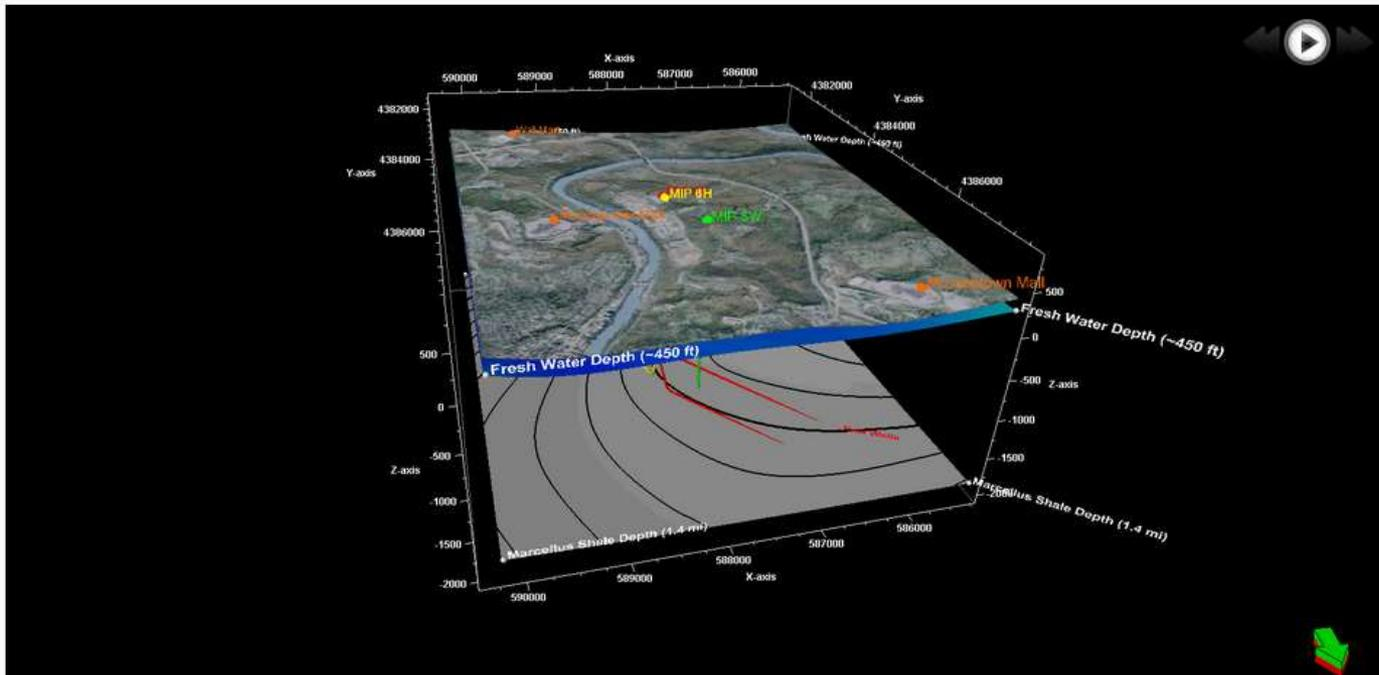
MSEEL site model shows the paths of the existing wells (yellow), new wells (red) and observation well (green) in relation to surface features and the bottom of the fresh water limit. The average fresh water depth is -450 ft beneath the surface. The depth of the Marcellus shale at 1.4 miles beneath the surface.
