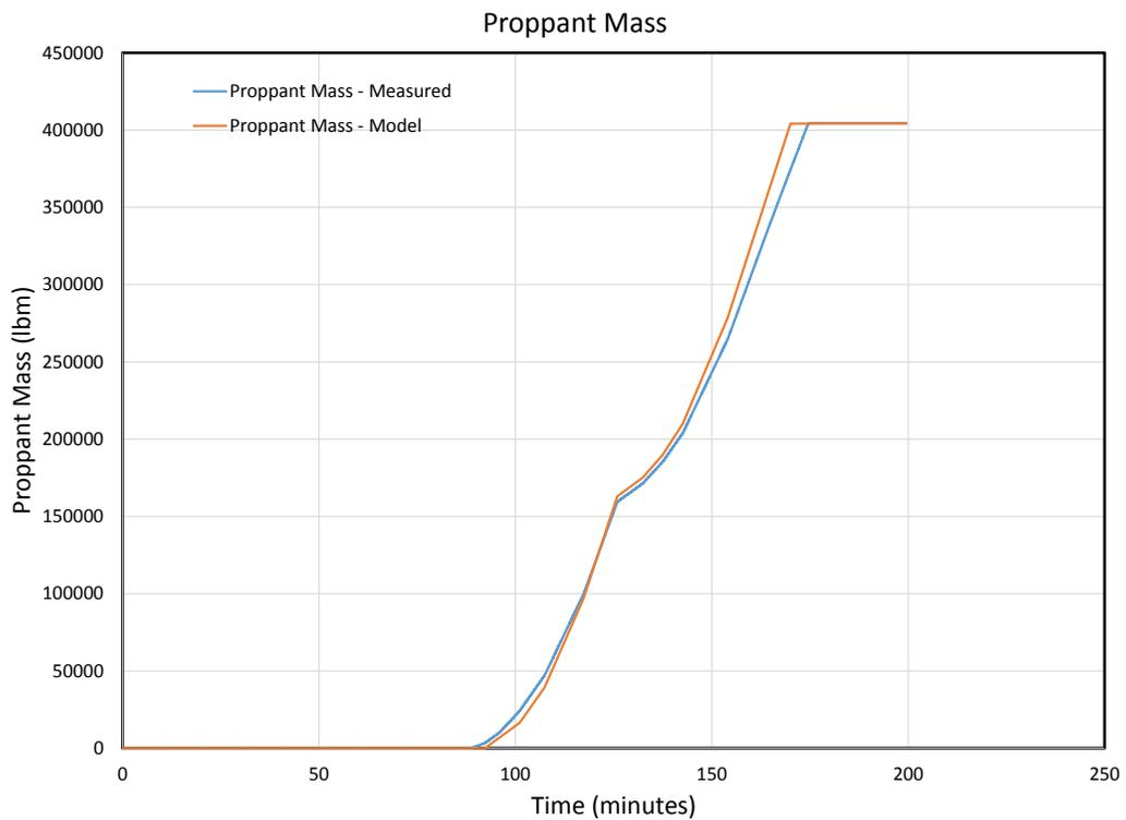
Figure 4.b.5: Proppant Mass vs Time for Stage 3 - MIP 3H
